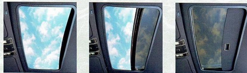
The sun, moon and stars are yours with Mark VII's optional power moonroof. Shown here open, partially closed and with sliding sun/shade panel extended.
