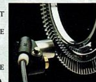
Mark VII's Anti-Lock Brake System begins with a speed sensor at each wheel that sends information to a microprocessor.
